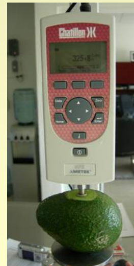
MEASURING SKIN AND PULP COLOR, FIRMNESS AND DRY MATTER
