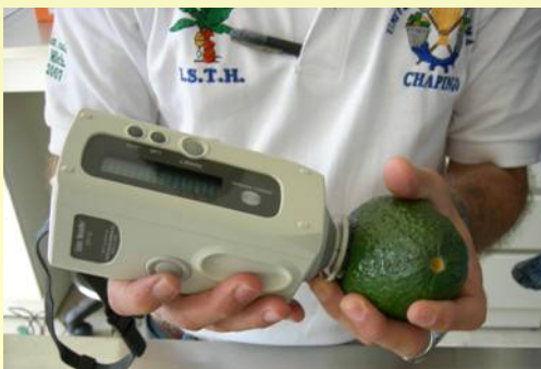
MEASURING SKIN AND PULP COLOR, FIRMNESS AND DRY MATTER
