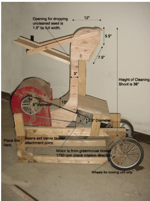
**Figure 2.** Seed cleaner constructed at WSU Vancouver REU.
